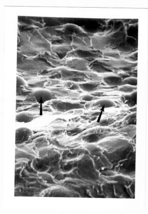
Photomicrograph of Duraflow acrylic resin processed by the conventional Compression Moulding Technique.  $(3mm \ thick, \ 300X, \ 10KV)$
