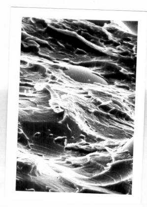
Photomicrograph of Leucitone acrylic resin processed by the Dry Heat-High Pressure Technique.
