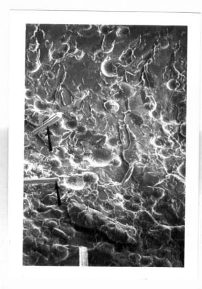
Photomicrograph of Leucitone acrylic resin processed by the conventional Compression Moulding Technique.
