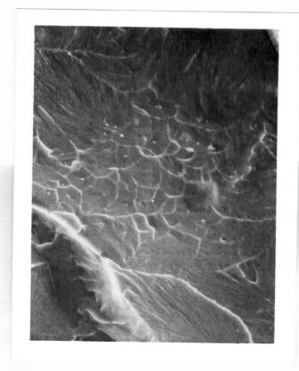
Photomicrograph of the Arnold acrylic resin processed by the Dry Heat-High Pressure Technique.
